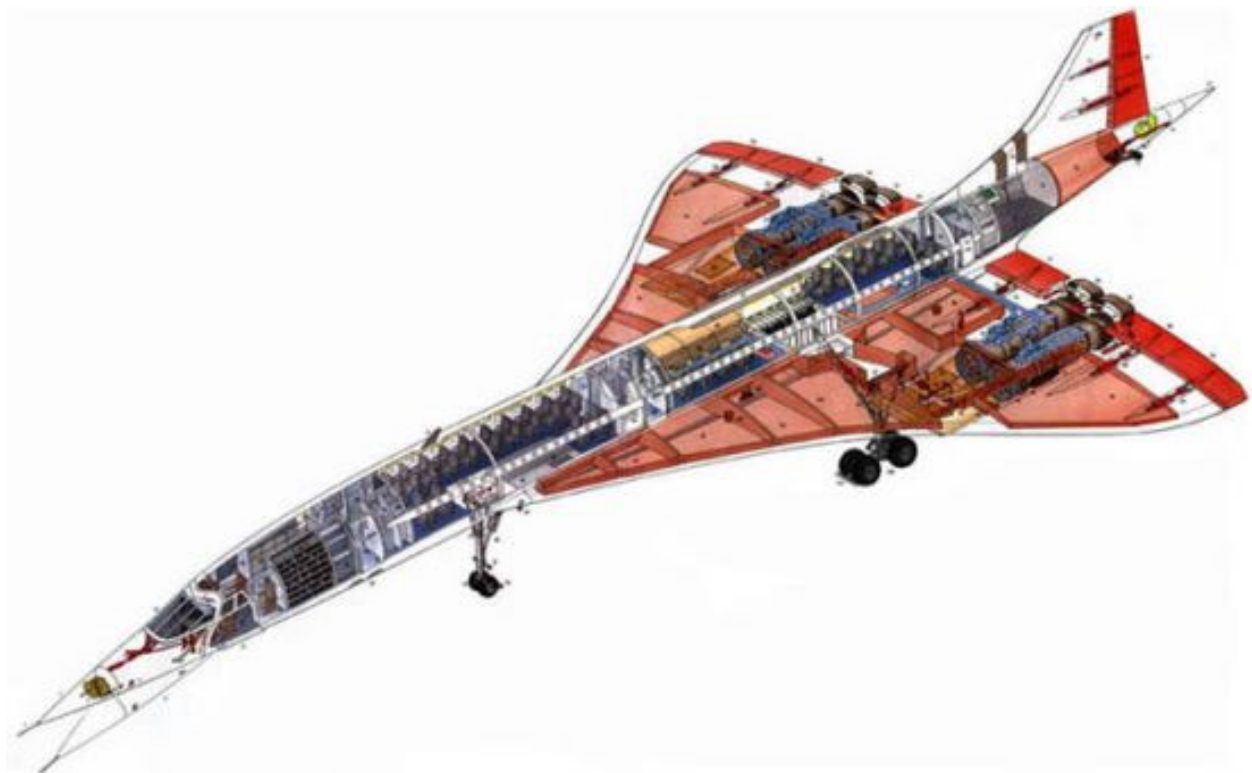
Figure 3: An internal schematic of the Concorde ix showing the fuel tanks, engines, and passenger chairs among other things. NOTE: The absence of a rear horizontal stabilizer.
